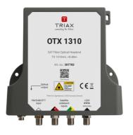
**The OTX 1310 SAT Fibre Optic Headend Kit** consists of the Wideband LNB TWB 40 and the OTX 1310 SAT FO Transmitter including the wall plug PSU. This headend enables to distribute the vertical and horizontal SAT widebands combined with terrestrial broadcast channels over a fibre optic (FO) network to a large amount of buildings and homes.
